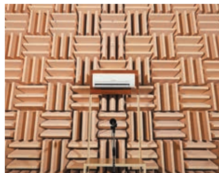
Anechoic Chamber Noise Test
